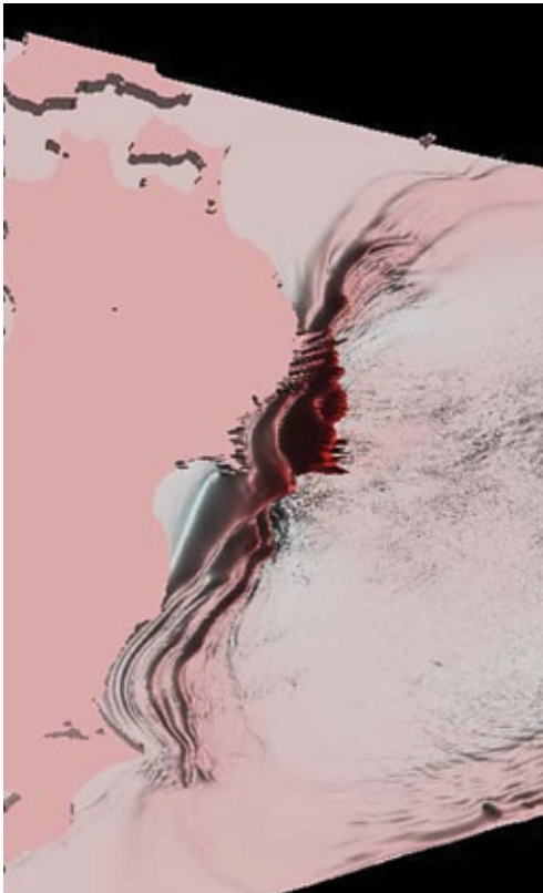
Fig. 1. Numerical computation of the 2011 Tohoku Tsunami (28 minutes after the earthquake)
